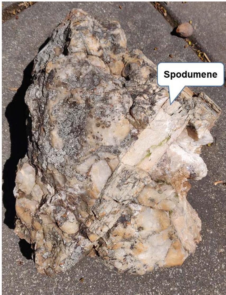
**Figure 2:** Coarse spodumene from Deep Purple pegmatite
