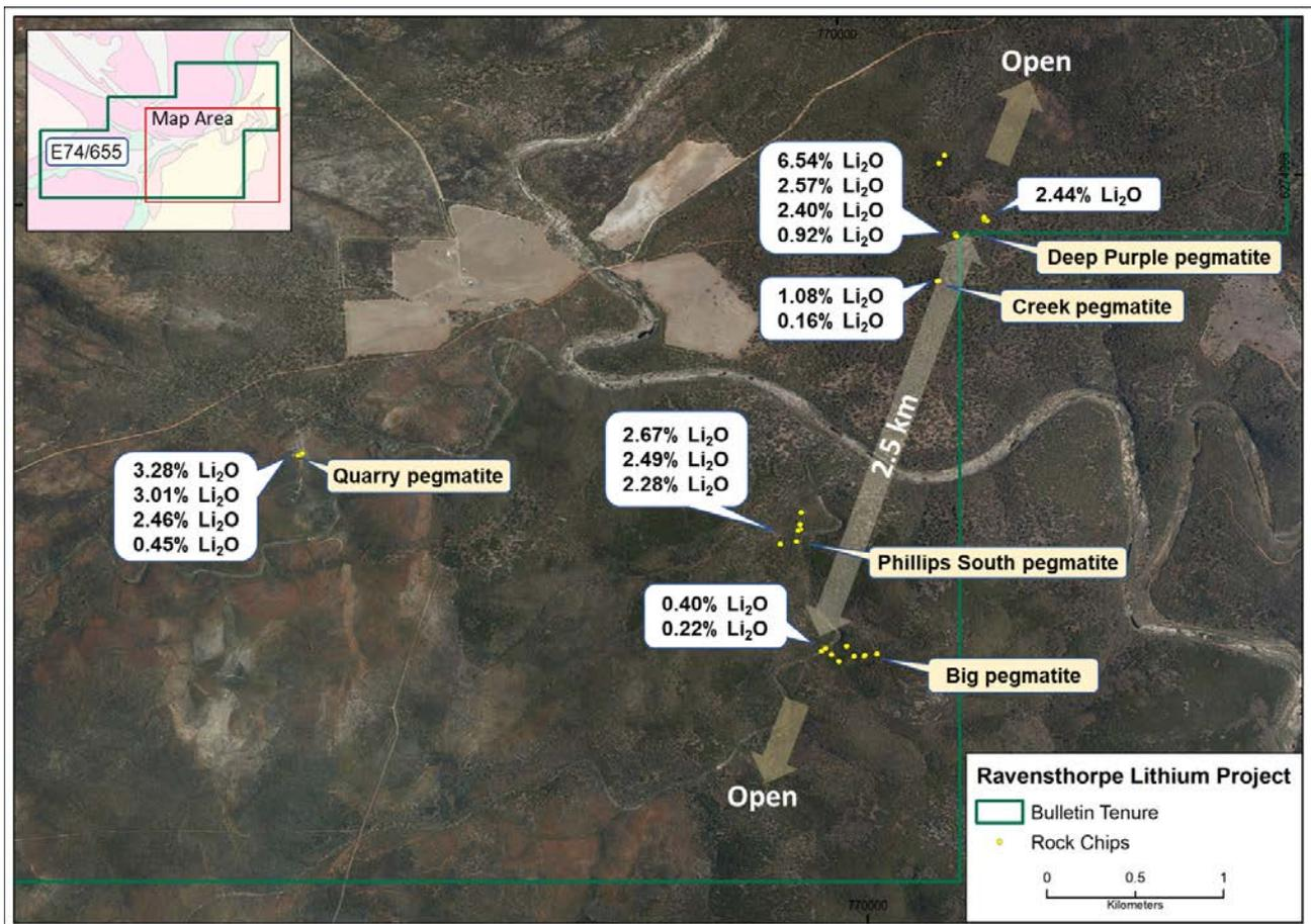
**Figure 1: Location and assays of rock chip samples above 0.2% Li<sub>2</sub>O**
